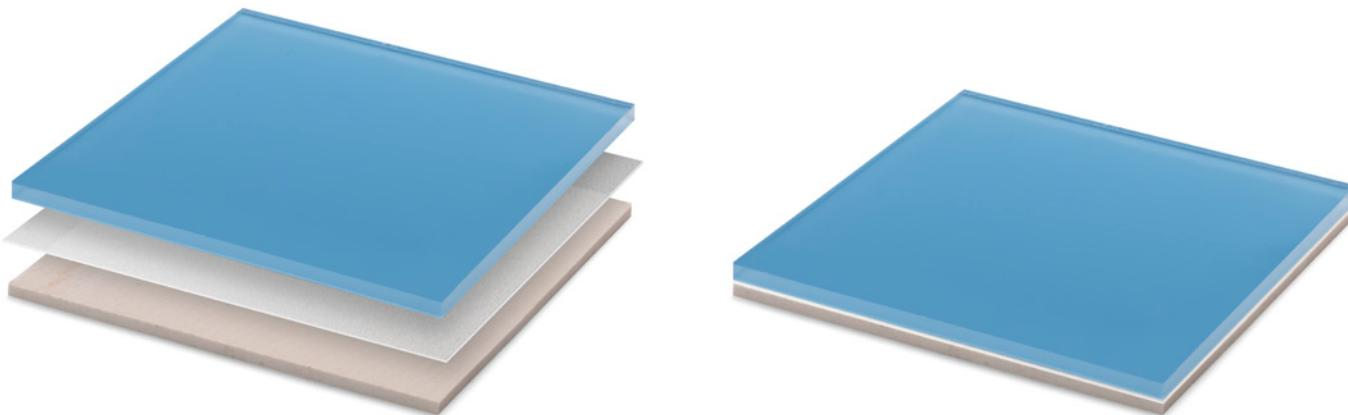
Covering formed by the stratified matching of a layer of 4mm of glass and a layer of 5mm of ceramic for a total thickness of around 10mm. Glasstile can be produced thanks to a process of high-temperature vacuum-sealing with a special sealant put between the ceramic and the enameled glass sheets that creates a single element. This new element is resistant to moisture and chemical agents and has customized finishes.
