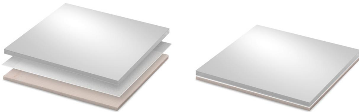
Covering formed by the stratified match of a layer of 5mm mirror and a layer of 5mm ceramic for a total thickness of around 11mm. Glass can be produced thanks to a technology that, with a process of high-temperature vacuum-sealing with a special sealant put between the ceramic and the glass sheets, creates a single element. This new element is resistant to moisture and chemical agents. This covering in SPECCHIO 02 finish is available in tiles of 100x100 cm and in customized sizes.
